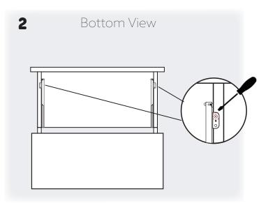
The runners are attached at the bottom of the drawer. Look for screws that hold the runner as circled in the picture. Use a screwdriver to unscrew the screws and remove them.
