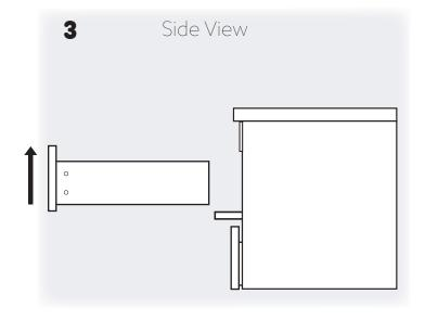
Once the release levers are disengaged, gently lift the drawer up and out of the cabinet.
