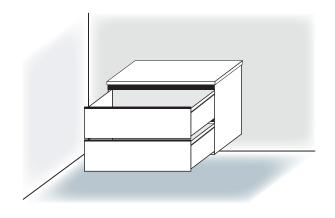
Install drawers and doors back onto the cabinet and make adjustments to align the doors and drawers correctly. Remember that it is the responsibility of the installer to make any adjustments to drawers and doors after installation. Don't forget to remove the transportation blocks on the underside of the cabinet.
